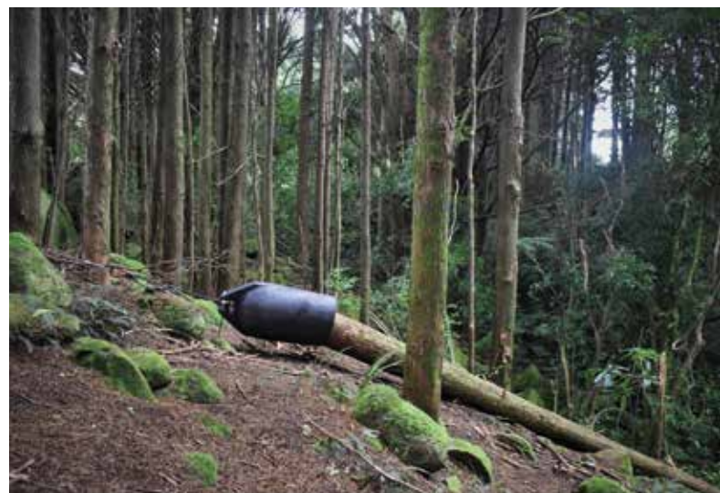
Figure 4: The D.I.Y. skidding cone proved its worth. The nose cone helped avoid snagging the logs on rocks, roots, humps and stumps, and minimised soil disturbance and damage to the forest
