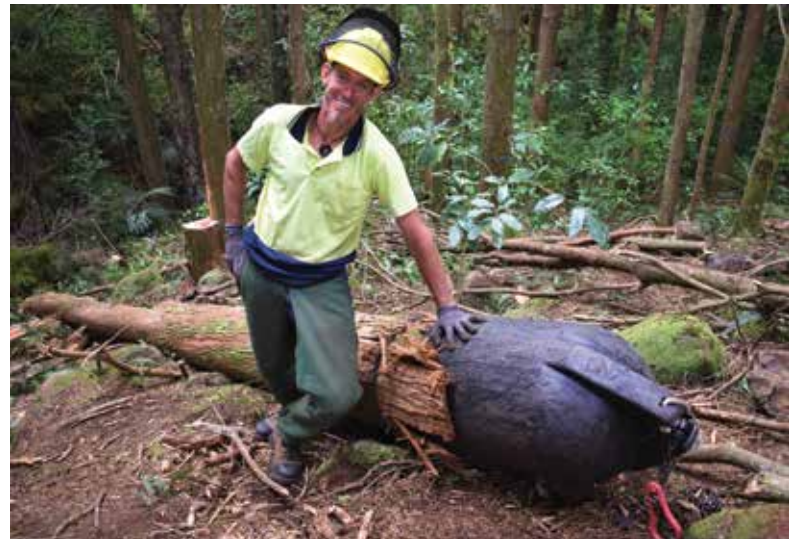
Figure 3: Ingenuity – Li Legler re-purposed a mussel farm buoy into a skidding cone
