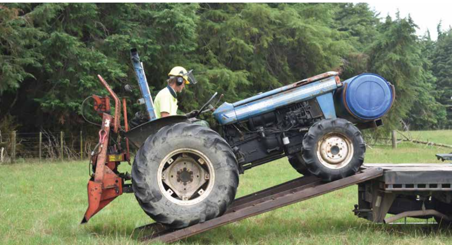
Figure 2: European-style forestry equipment – a 45-horsepower tractor with a PTO-driven winch on the 3-point linkage and a 4-tonne pulling capacity
