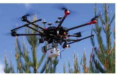
Figure 2: Scion unmanned UAV collecting LiDAR data over a pine forest
