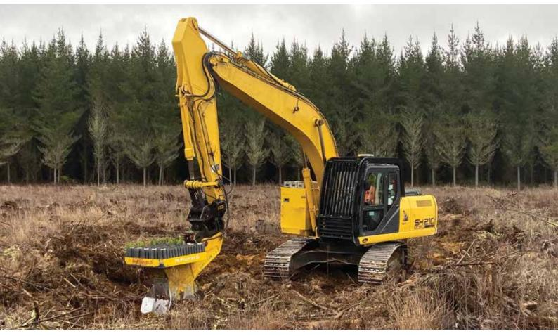
Figure 8: M-Planter in Kinleith Forest, Tokoroa. Multiple companies in NZ are currently using mechanised planting machines
