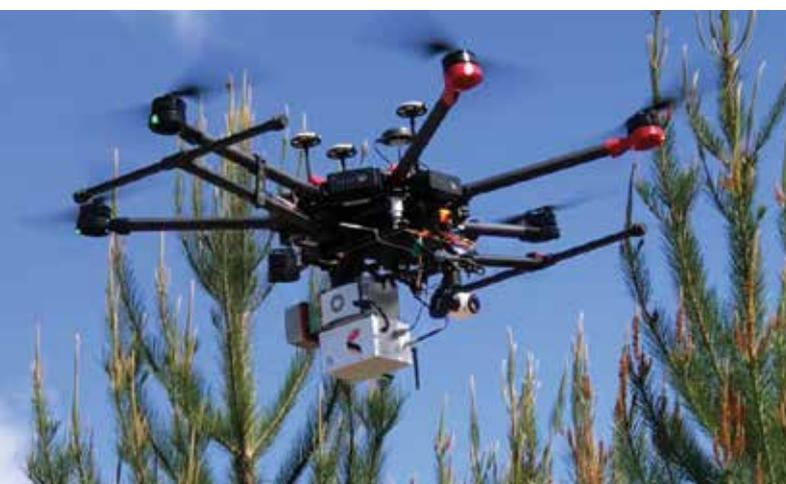
Figure 2: Scion unmanned UAV collecting LiDAR data over a pine forest
