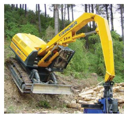
Figure 10: ClimbMAX Steep Slope Harvester manufactured by Trinder Engineers Ltd, Nelson (the first commercial NZ-made winch-assisted harvester)
