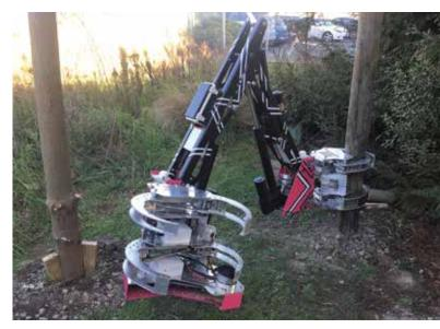
Figure 9: An example of a smaller machine – a robot capable of moving from tree-to-tree to carry out forest thinning operations developed in collaboration with Scion scientists, FP Innovations and inFact Ltd
