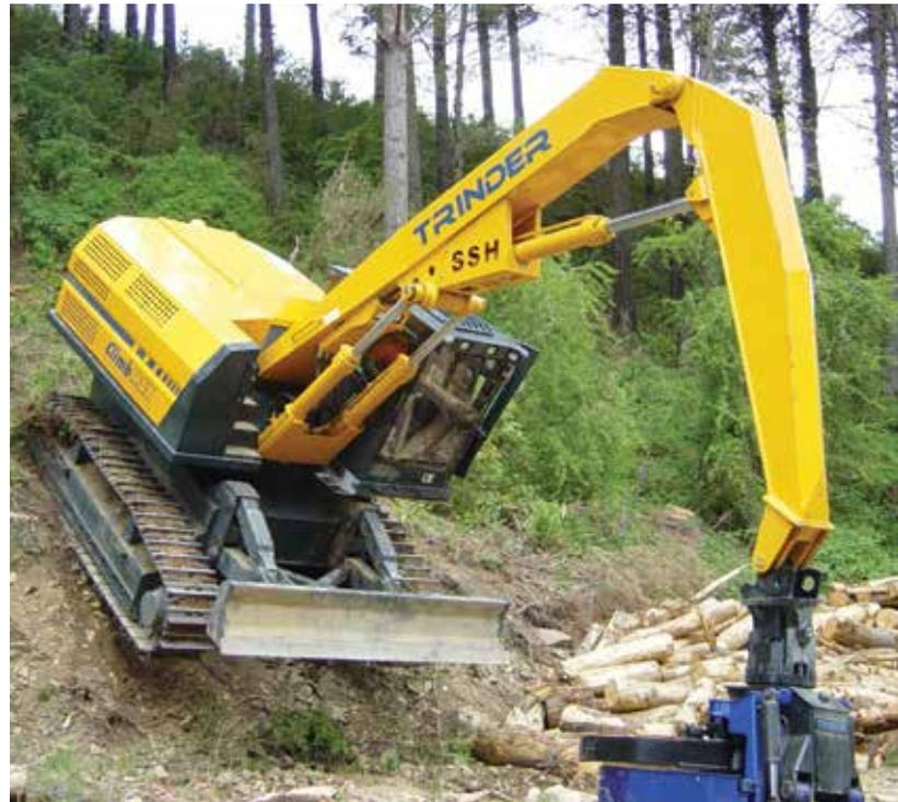
Figure 10: ClimbMAX Steep Slope Harvester manufactured by Trinder Engineers Ltd, Nelson (the first commercial NZ-made winch-assisted harvester)
