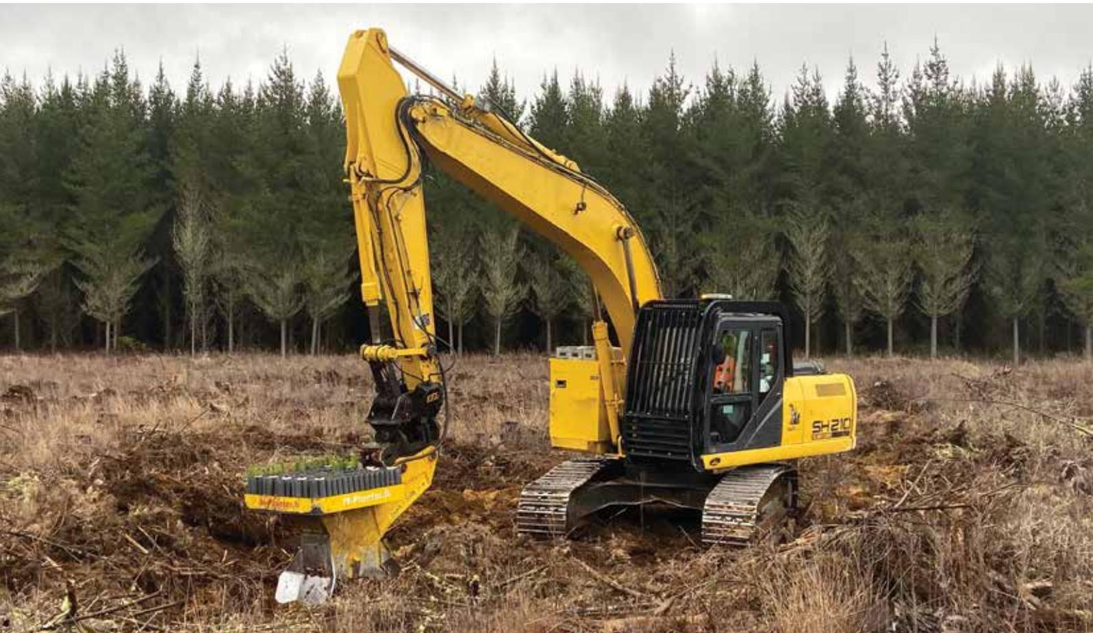
Figure 8: M-Planter in Kinleith Forest, Tokoroa. Multiple companies in NZ are currently using mechanised planting machines
