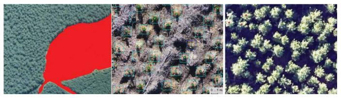
Figure 4: Deep learning (AI) models have been shown to work well for tasks such as mapping cutover (left), detecting seedlings (centre) and counting individual trees after thinning (right)
