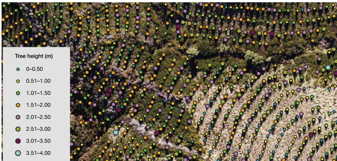
Figure 7: AI-derived tree locations and heights from fixed-wing aerial imagery (5 cm)
