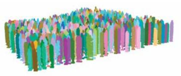
Figure 6: UAV LiDAR point cloud colourised by individually segmented trees
