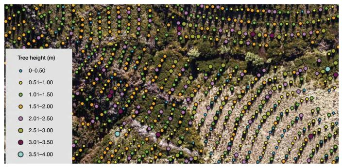
Figure 7: Al-derived tree locations and heights from fixed-wing aerial imagery (5 cm)
