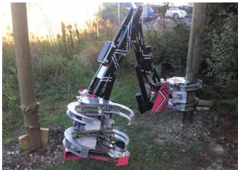
Figure 9: An example of a smaller machine – a robot capable of moving from tree-to-tree to carry out forest thinning operations developed in collaboration with Scion scientists, FP Innovations and inFact Ltd
