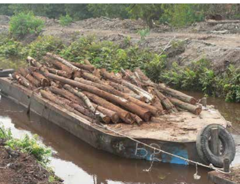
Small barge used for transporting logs from the harvesting site to a log yard
