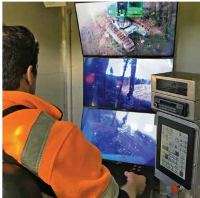
Operator console for teleoperation of the feller buncher
