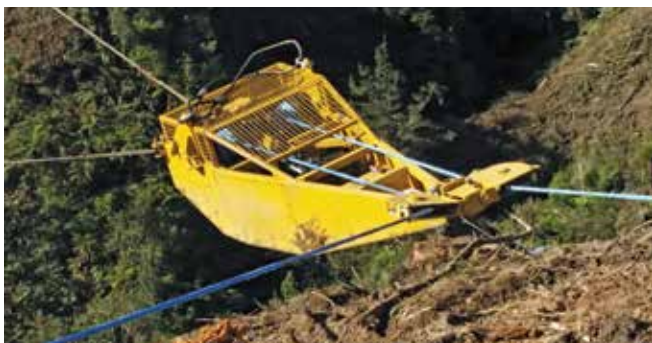
Skyshifter remote-controlled tail-hold carriage
