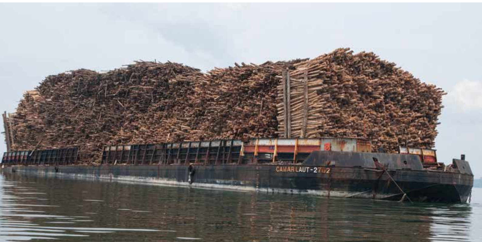
Large ocean-going barge for inter-island log transport
