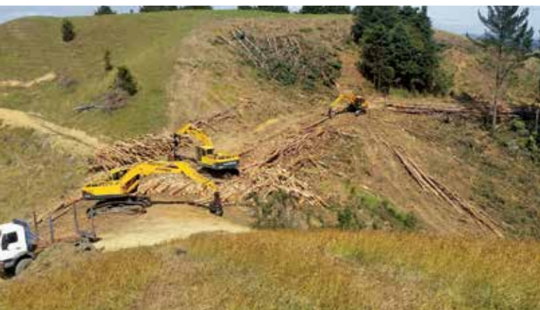
Bent Fish Gully with the processing machine in the centre. An off-road truck loading machine is temporarily shovelling in the background. The felling machine has been shovelling from the right (out of picture) and is about to load an off-road truck which is reversing into position
