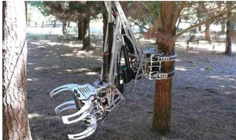
Figure 5: Prototype autonomous harvesting system developed by Scion and the University of Canterbury. Photo courtesy of Richard Parker, Scion
