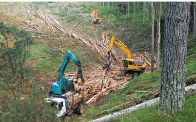
At the Basin, a felling machine is in the background and shovelling to feed the processor. A processing machine is in the centre working atop a waste pile. An off-road truck is being loaded in the foreground
