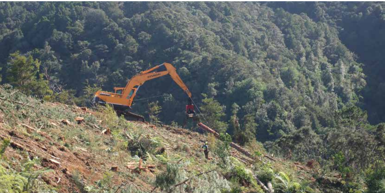
30 tonne excavator fitted with a chainsaw felling head and winch. The trees are felled manually with winch assist and are pulled up the hill and picked up by a grapple. The Taheke Scenic Reserve (DOC) is in the background
