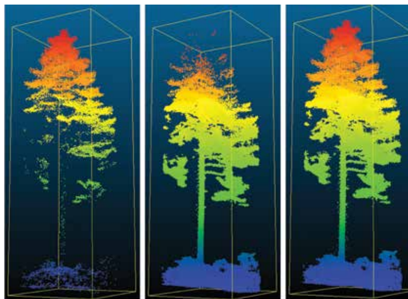
Figure 2: Laser scanning results for an individual tree. (Left) scanned from above; (middle) scanned from below; (right) composite image
