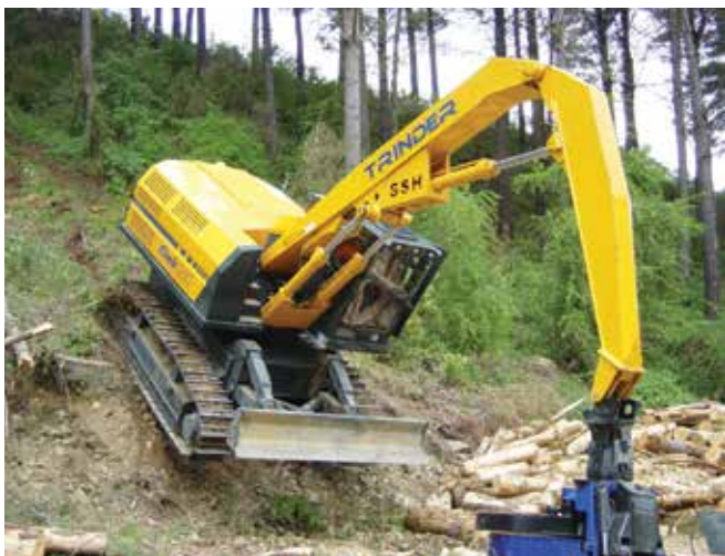
Winch-assisted felling with the ClimbMAX steep slope harvester
