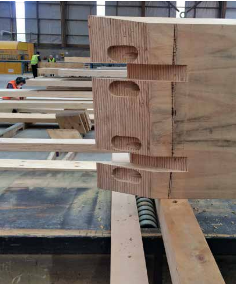
Detail of CNC shaping to LVL beam for housing metal bracket connections
