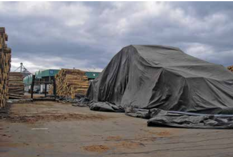
Pinus radiata logs being treated under cover with methyl bromide prior to export
