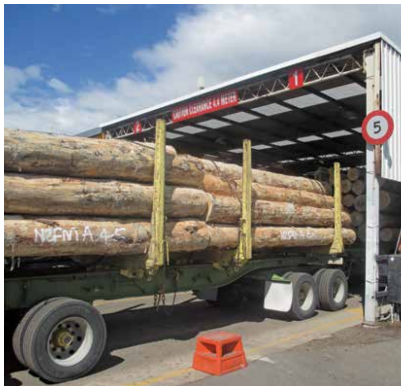
Pinus radiata logs that have been processed with a mechanised processor can end up with less than half of the bark remaining – in this case almost all of the bark has been removed
