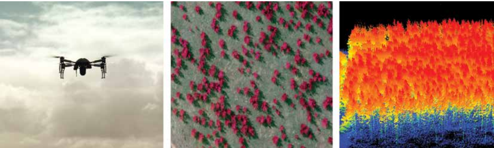
Figure 4: A multi-rotor UAV similar to the device developed for Scion by Aeronavics Ltd that will provide a platform for research into precision forestry and samples of 5-band multi-spectral imagery and ALS data acquired with the device. The multi-spectral image shows wilding pines visible in purple, the ALS image shows a dense point cloud collected over a mature radiata plantation in the Bay of Plenty. Photo: Aeronavics Ltd, Scion
