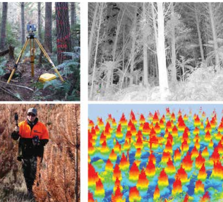
Figure 2: A tripod mounted (top) and mobile laser scanner (bottom) being used by Scion's researchers in New Zealand's forests with examples of the point clouds generated. Photos: Rod Brownlie
