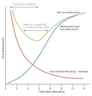
Figure 1: An example of typical changes in forest vegetation root strength or root reinforcement after timber harvesting showing the 'window of vulnerability' (see Phillips et al. 2012 for more details)
