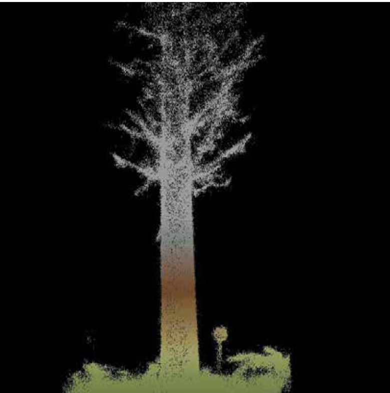
Figure 3: Terrestrial LiDAR image of a standing tree captured using the ZEB1 instrument. Source: Courtesy of Rod Brownlie, Scion
