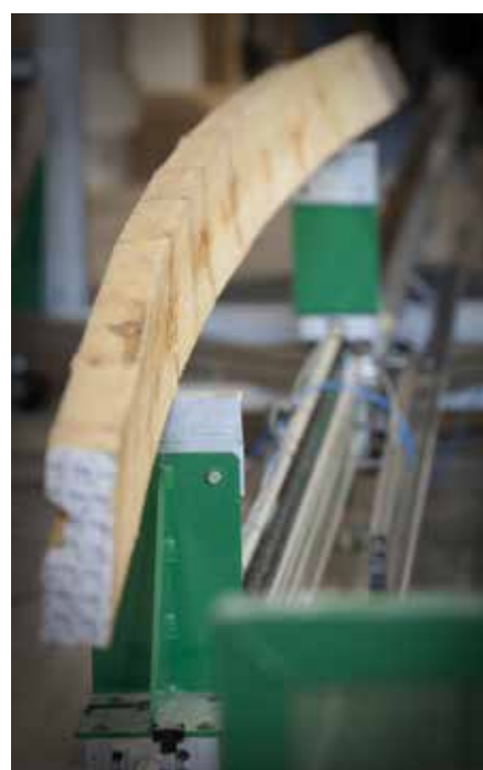
Example of intra-ring checking in a radiata pine moulding. Source: Scion Digital Image Library
