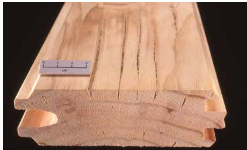
Example of intra-ring checking in a radiata pine moulding. Source: Scion Digital Image Library
