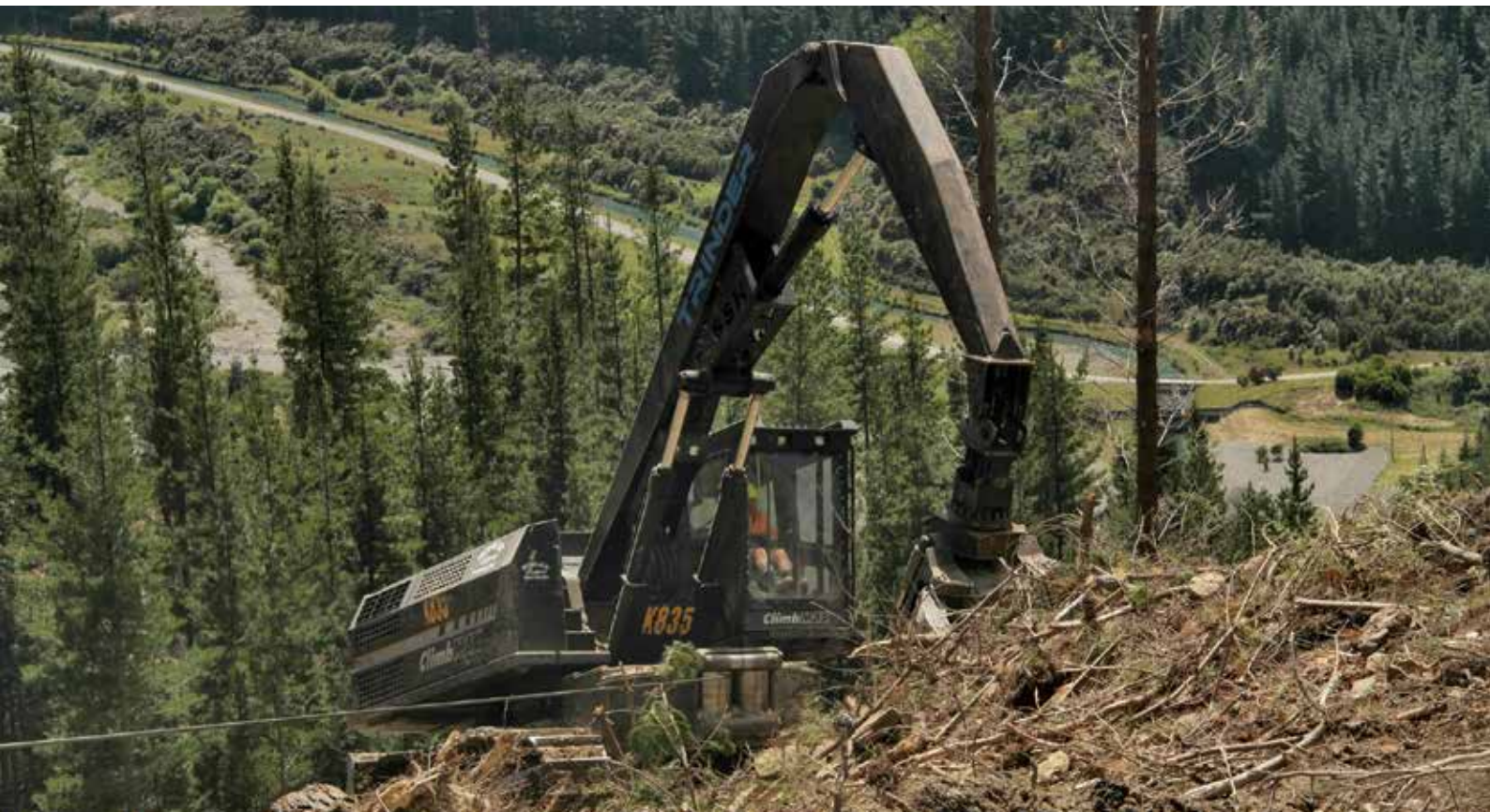
ClimbiMAX felling machine with winch integrated into chassis
