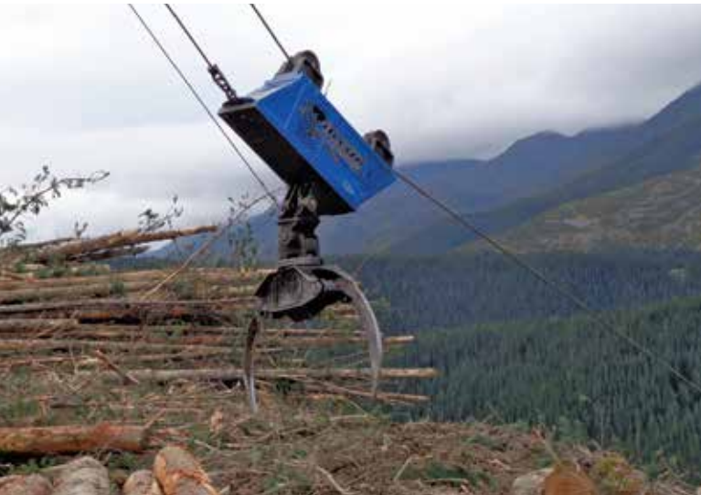
Motorised grapple carriages – Falcon Forestry Claw with internal motor (left) and hydraulically-powered Alpine (right)
