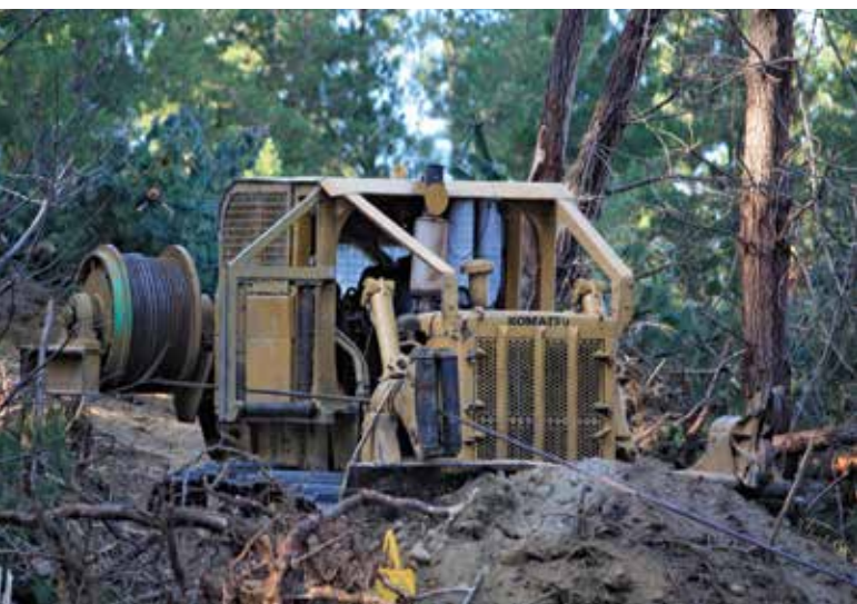
Purpose-built self-levelling harvester (right) being cable-assisted by the winch mounted on the dozer (left)
