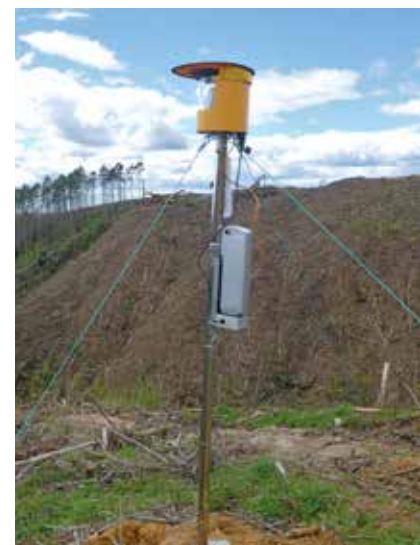
Camera mounted into a mechanical grapple carriage (left) and camera mounted in the cutover (right). Both cameras transmit a video signal back to the yarder cab to assist the operator with the grappling task
