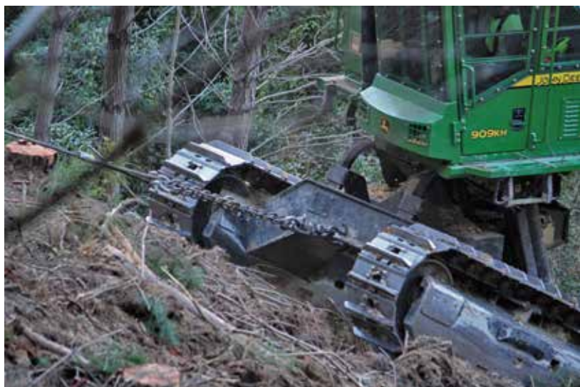
Purpose-built self-levelling harvester (right) being cable-assisted by the winch mounted on the dozer (left)
