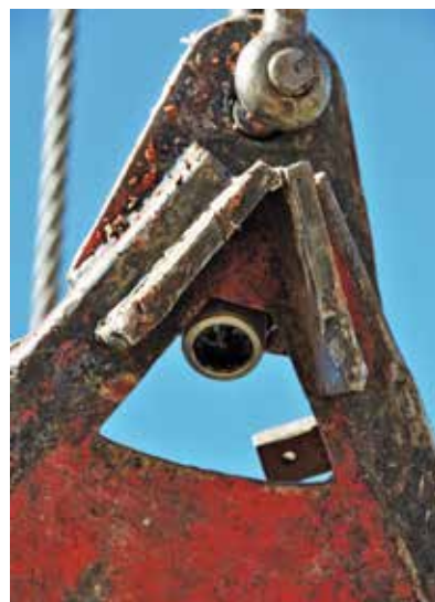
Camera mounted into a mechanical grapple carriage (left) and camera mounted in the cutover (right). Both cameras transmit a video signal back to the yarder cab to assist the operator with the grappling task
