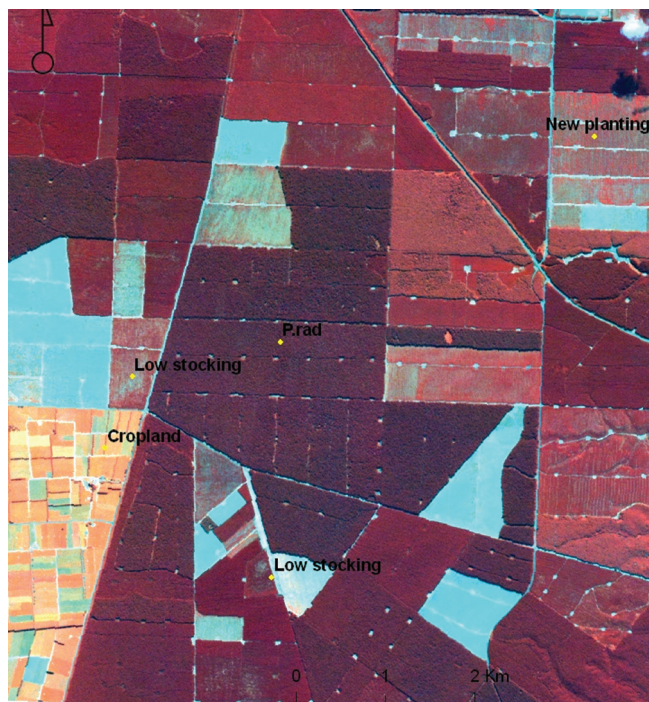
Figure 5. Processed RapidEye image showing the area described in figure 3 using a false colour composite that includes the near infrared band. The use of the near infrared band assists in highlighting the differences in crop vigour.
