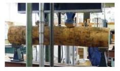
Walford and Chapman (pp. 83-90) found that stress-wave velocity was more effective than basic density of outer-zone wood for selecting *Pinus radiata* poles for structural uses. A minimum stress-wave velocity reading of 2.8 km/s is recommended. The authors conclude that New Zealand Standard3603 should be amended in the light of these findings.
