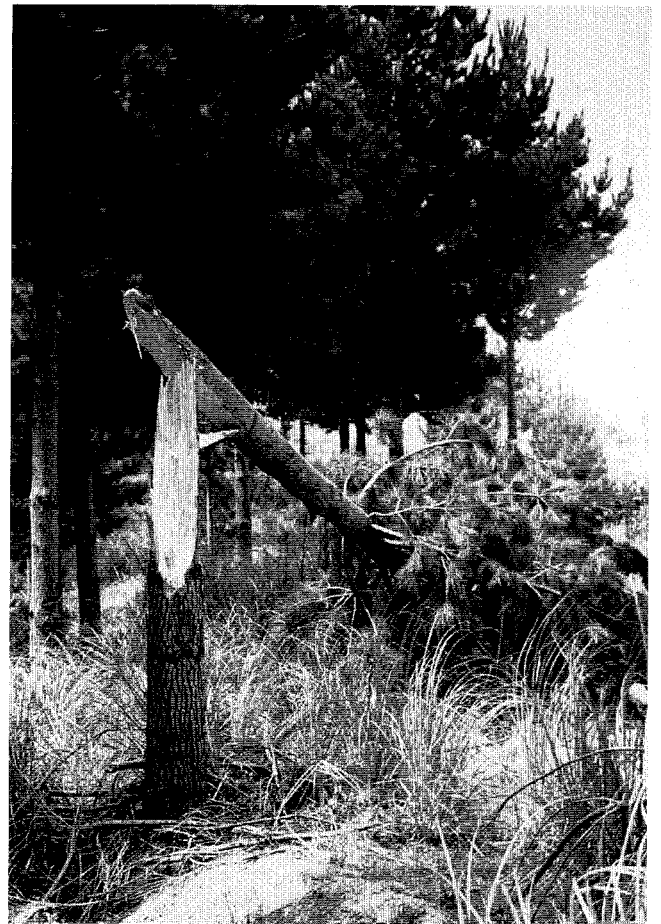
Tree winched over at Maramarua Forest which has failed by stem fracture. Photo: John Moore
