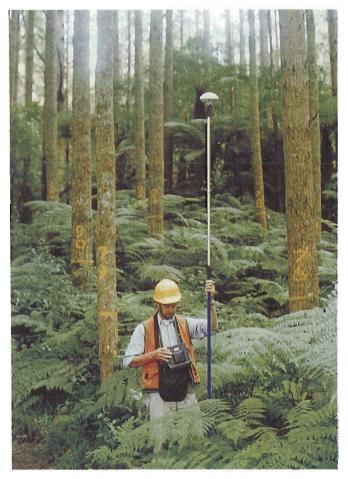
Figure 1. Evaluating a GPS unit to record the location of a sample plot in a forest stand.
