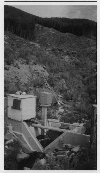
A stream gauging weir and sediment trap on a radiata pine stream in the Marlborough Sounds. This installation is part of a long-term experiment to evaluate the impacts of clearfelling radiata pine forest on stream water quantity, quality and sediment yields. Photo: Landcare
