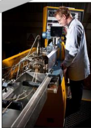
Lab scale extruder (~20kg/h)
