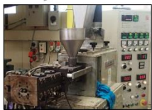
Bench scale extruder (~1kg/h)
