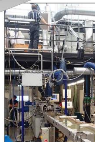
Pilot scale extruder (~150kg/h)
