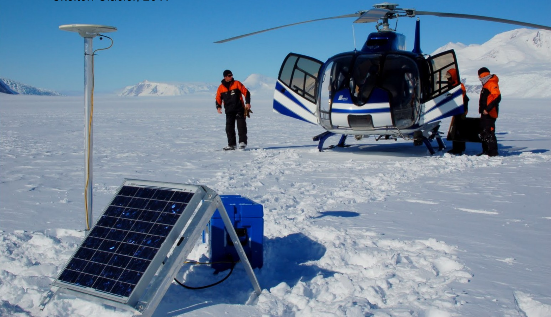
Ice velocity GNSS survey, Skelton Glacier, 2011
